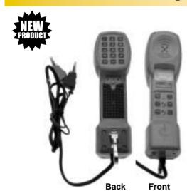
**Uses:** Used by installers and repair technicians for line testing and temporary communications.
