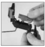
Blade height adjustment gauge. Allows easy adjustment for most common cable sizes. Included in all full kits.
